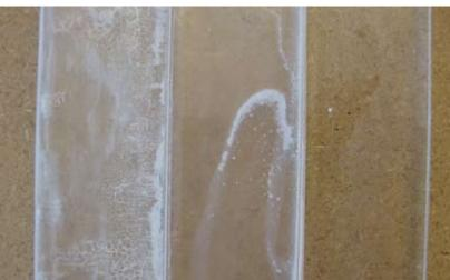
Three lightguides with 3, 2, and 1 coat(s) of 1:3 TPB to polystyrene coating.
